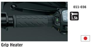
57100-06824-000 Heats the entire surface of the grips and offers three different level settings to keep hands warm when riding in cold weather.
