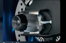
99116-48K00-000 Helps reduction of damage, made of aluminium
