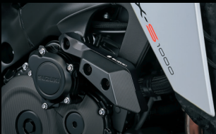
Frame slider Helps reduction of damage, made of aluminium and ertacetal.
