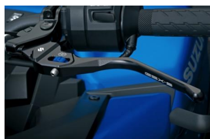
11 Billet clutch lever (Anodized) Made of high-end billet aluminum
