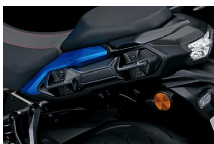
4 Side case bracket set For attaching side case set In combination with side case set
