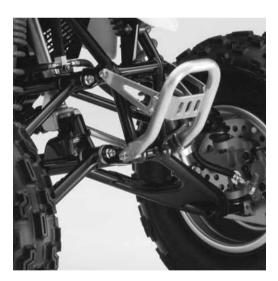
■ Piggyback-reservoir shock absorbers front and rear (carried over from current model)
