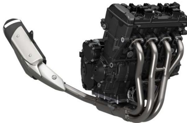
We chose to use the 2005 GSX-R engine as a base rather than the unit from the current GSX-R750 because its engine mounting angle is close to vertical. This helps realise the short wheelbase wanted on a naked model.
