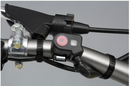
S-HAC switch and indicator light (located on the left handlebar)
