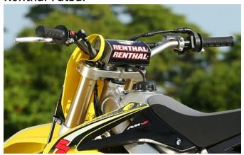
Renthal Aluminum Fatbar® is standard equipment. It has more strength and less vibration than aluminum straight handlebars.
