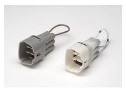
For quick fuel adjustment setting to suit riding condition, two couplers are enclosed. One is for rich and another for lean fuel setting compared to stock setting. Customer can change fuel setting to best suit the riding conditions by just connecting either coupler.
