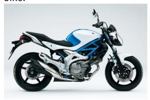
These lightweight sport roadsters are powered by 90-degree V-twin engine. In today's 600-700cc class, models from other brands are mostly powered by parallel two or four cylinder engine. The reason why Suzuki keeps offering the V-twin roadster is, we value the uniqueness that only V-twin engine can offer.
