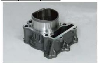
SCEM (Suzuki Composite Electrochemical Material)-plated cylinders reduce friction and improve heat transfer and durability.
