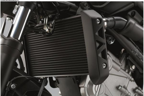
> The Newly designed, high-efficiency radiator with enlarged cooling fan; has strong cooling performance.
