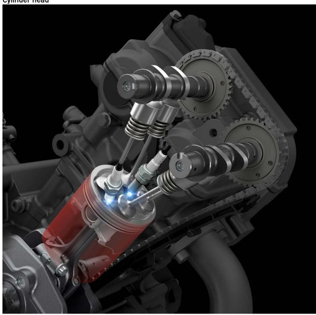
➤ The cylinder heads feature Suzuki's original Dual Spark Technology for greater combustion efficiency, better fuel economy and cleaner emission.
