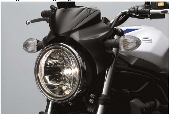
Round shaped headlight is multi-reflector type with 12V60/55W bulb.
