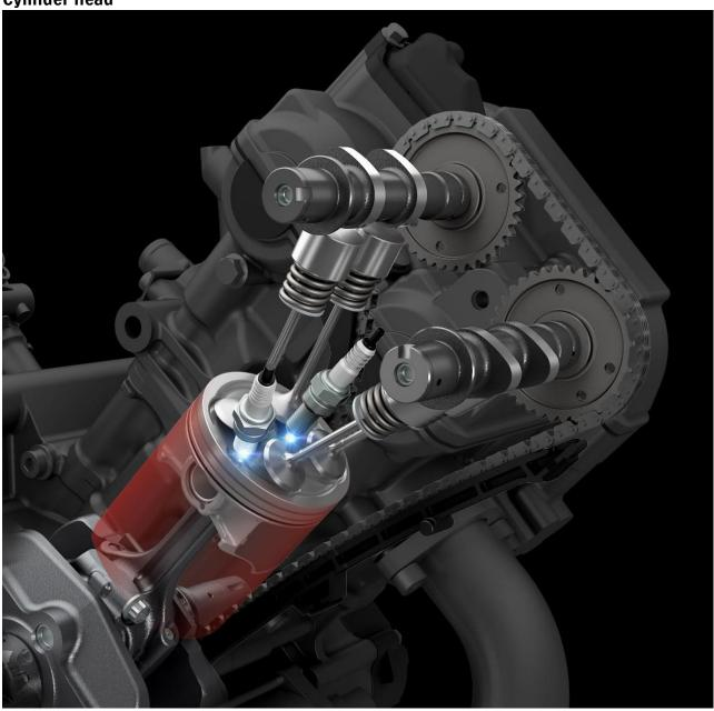
> The cylinder heads feature Suzuki's original Dual Spark Technology for high combustion efficiency, fuel economy and clean emissions.
