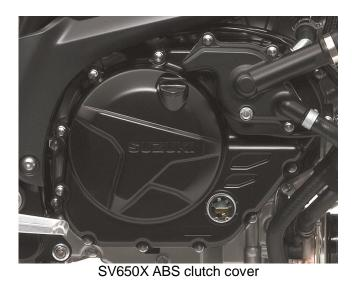
> Clutch cover is designed to reduce weight.
