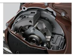
Suzuki Assist Clutch System (SACS)
